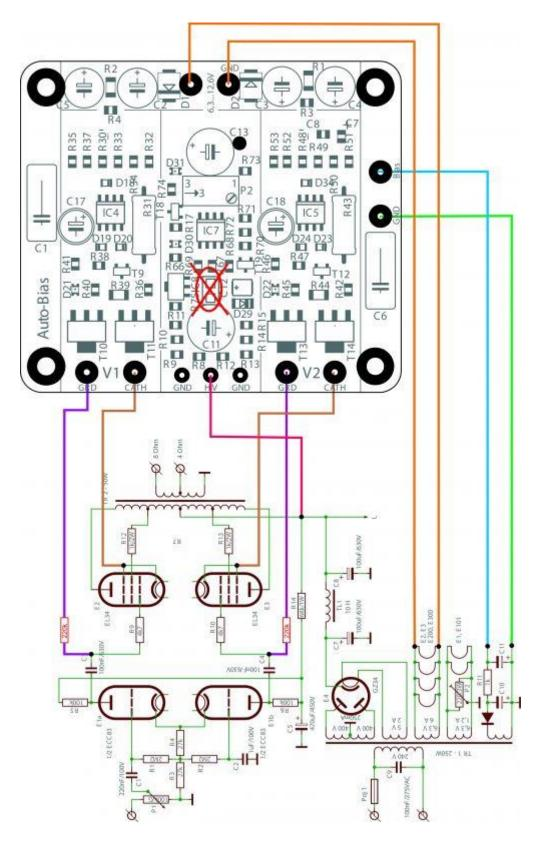
The circuits of the first grids of the output tubes must be equipped with isolation resistors (marked red with the value 100-220k).
