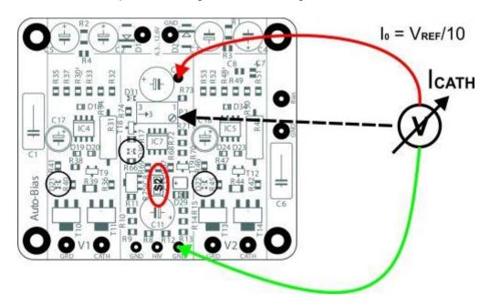
As a rule, S2 jumper on the module serves to connect the local source for generating the reference voltage. If the reference voltage is to be taken from the anode supply voltage (in case of a delayed ramp up of the anode voltage, for instance), apply this voltage to HiV and disconnect the S2 jumper.
