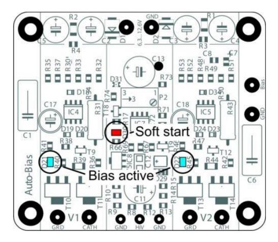
After the module has been connected and the AC supply voltage of 6.3 ...12.6V applied, the "Soft Start" function will be initiated. The red LED located in the reference part of the module (Soft start) will be on for about 20 sec.
